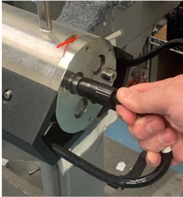
Figure 7-2: Aft Endcap Cable Disconnection
