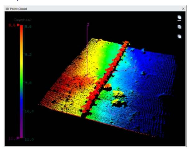
Profiling mode allows you to view a real-time 3D point cloud of the sea bottom or structures under the water. The profile point data can be exported to a file so that third-party software can extract depth, distance, and volume measurements.
