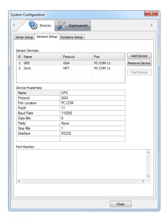
If you have external sensors that provide speed, heading, or latitude/longitude coordinates, then this dialog box allows you to set them up. Readings from these sensors will appear in the **Information Widget** located in the sonar view.
