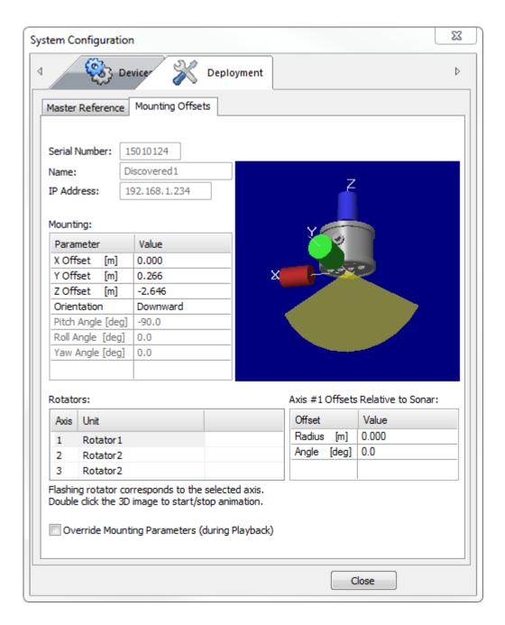
If you are mounting your M3 Sonar Head (on a Pole Mount for example), you will need to specify where the Sonar Head is positioned in three-dimensional space relative to the GPS antenna.
