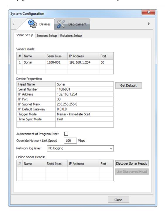
This dialog box allows you to connect to the Sonar Head. You can connect manually or automatically each time you start the software. This dialog box also provides diagnostic network tools.
