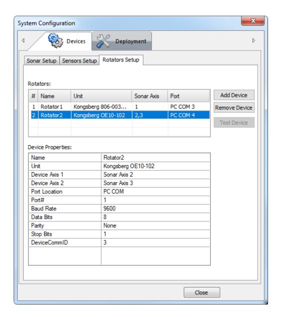
The M3 software supports the following rotators.
