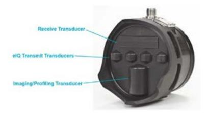
The Sonar Head includes transmit and receive transducers and the electronics to generate the transmit pulse and digitize the received signal. The sonar data is sent to the Sonar Processor using a standard Ethernet link.
