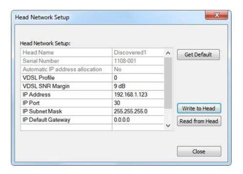
You can program the IP address and the IP port of the Sonar Head for various network environments. The factory default IP address is 192.168.1.234, and the default port number is 30.
