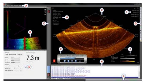
The presentation provides you with a lot of information. The sonar view presents sonar echo data. The 3D Point Cloud presents profile point data that can be rotated in three dimensions. The menu system on the top gives you easy access to all the functionality offered by the M3 software. The tool bar provides buttons for functions, filters, and sonar view overlays. The bottom **Output Messages** window and bottom status bar provide diagnostic messages.
