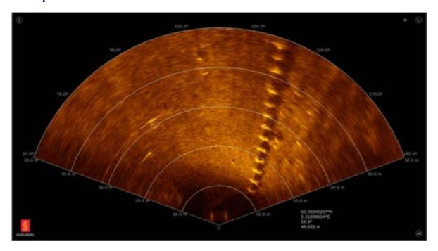
The range and bearing or X/Y coordinates of the current mouse cursor position is shown at the bottom of the sonar view.
