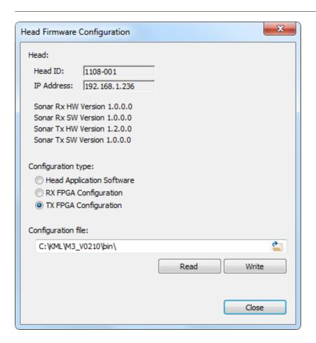
In addition to head application software, the Sonar Head has receive firmware (RX FPGA) and transmit firmware (TX FPGA). You can upgrade these by selecting the configuration type, browsing for the file, then clicking the **Write** button.
