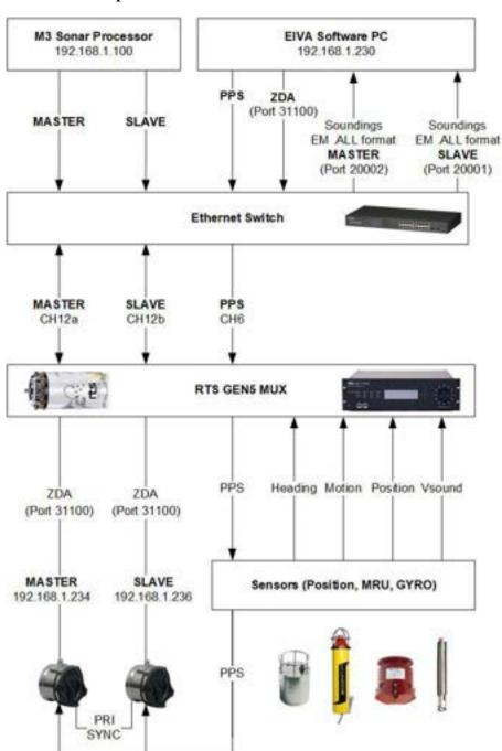
Dual M3 Sonar Setup using the ROV survey MUX and exporting data to the EIVA NaviSuite computer
