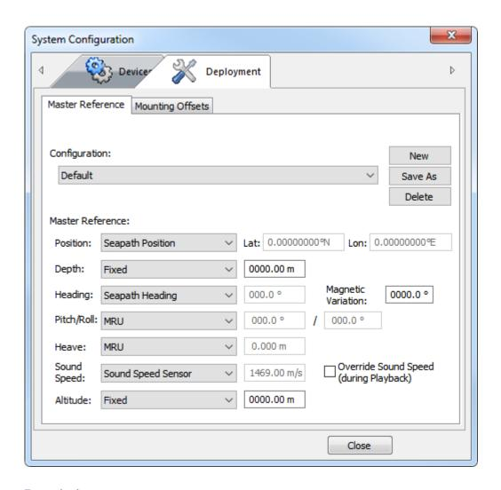
When using the M3 Sonar for imaging, set up sensors for **Position** and **Heading** if you want to create GeoTiff files or create a real-time mosaic.
