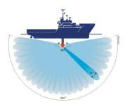
The HiPAP® 501 has a full spherical transducer body including 241 transducer elements. This model has close to full accuracy in the half sphere sector and is the preferred system where the best possible performance is required. The HiPAP® 501 can also track targets above the half sphere sector.
