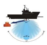
The HiPAP® 101 has a planar transducer array with a cylindrical body including 31 transducer elements. This model has good accuracy in the  $\pm$  60° coverage sector and is suited for operations where the major positioning targets are within this sector.
