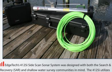
EdgeTech's 4125i Side Scan Sonar System was designed with both the Search & Recovery (SAR) and shallow water survey communities in mind. The 4125i utilizes EdgeTech's Full Spectrum® CHIRP technology, which provides higher resolution imagery at ranges up to 50% greater than non-CHIRP systems operating at the same frequency. This translates into more accurate results and faster surveys, thus cutting down on costs.
