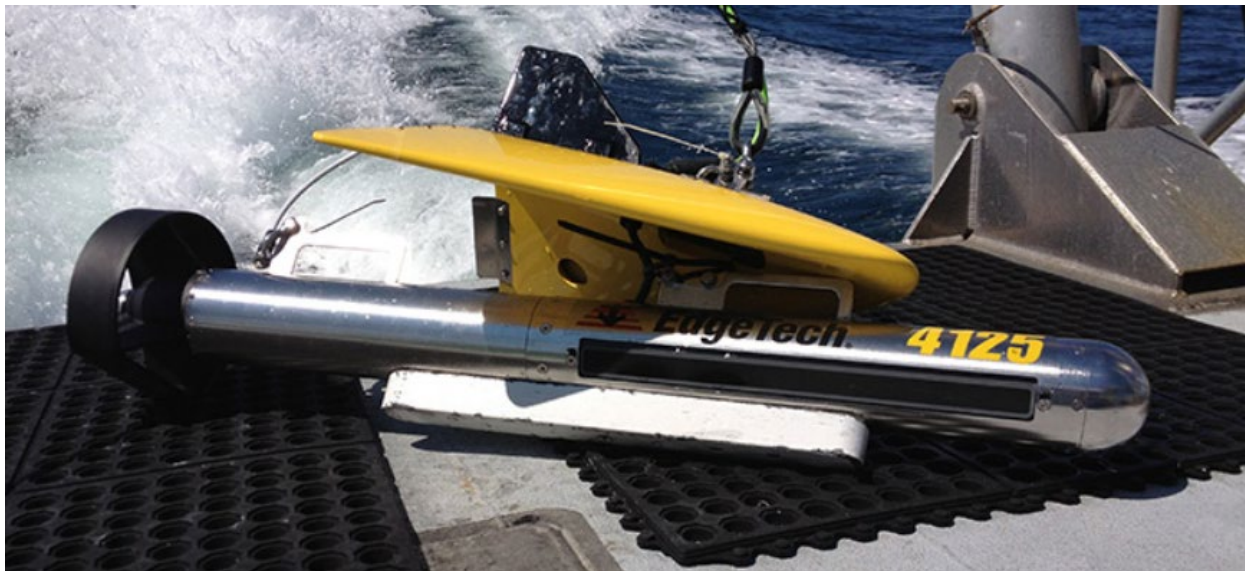
Figure 1-7: 4125 With Depressor Wing and Keel Weight Kits Installed
