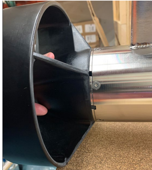
Figure 3-8: 4125i Tail Assembly Seating
