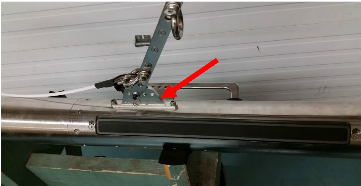
Figure 3-12: Vertical Hull-Scan Bracket Attached
