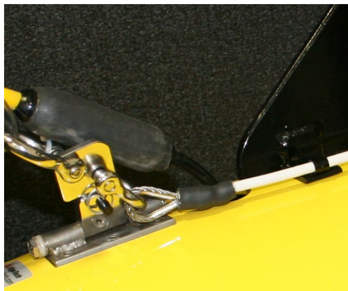
Figure 3-16: Tow cable shown Routed through Depressor Wing Top Hole.
