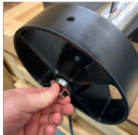
Figure 3-10: Tail Assembly Bolt Installation
