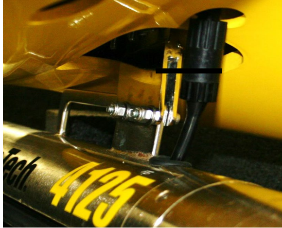
Figure 3-17: Tow cable and Tow Fish Pigtail Connectors.
