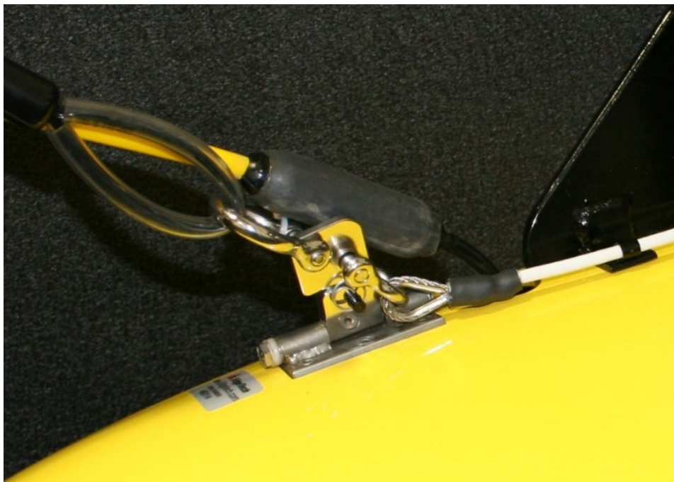
Figure 3-18: Cable grip attached to Depressor Wing Mounting Point.
