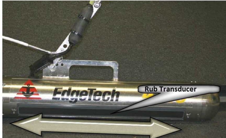
Figure 3-21: Performing a Rub Test
