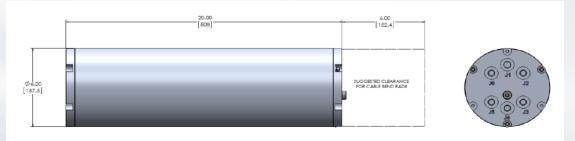
EdgeTech 2205 systems are available in a variety of configurations including 3,000 (shown above) and 6,000 meter rated pressure housings or electronics-only versions for installation in customers vheicle electronics sections. Call for details.
