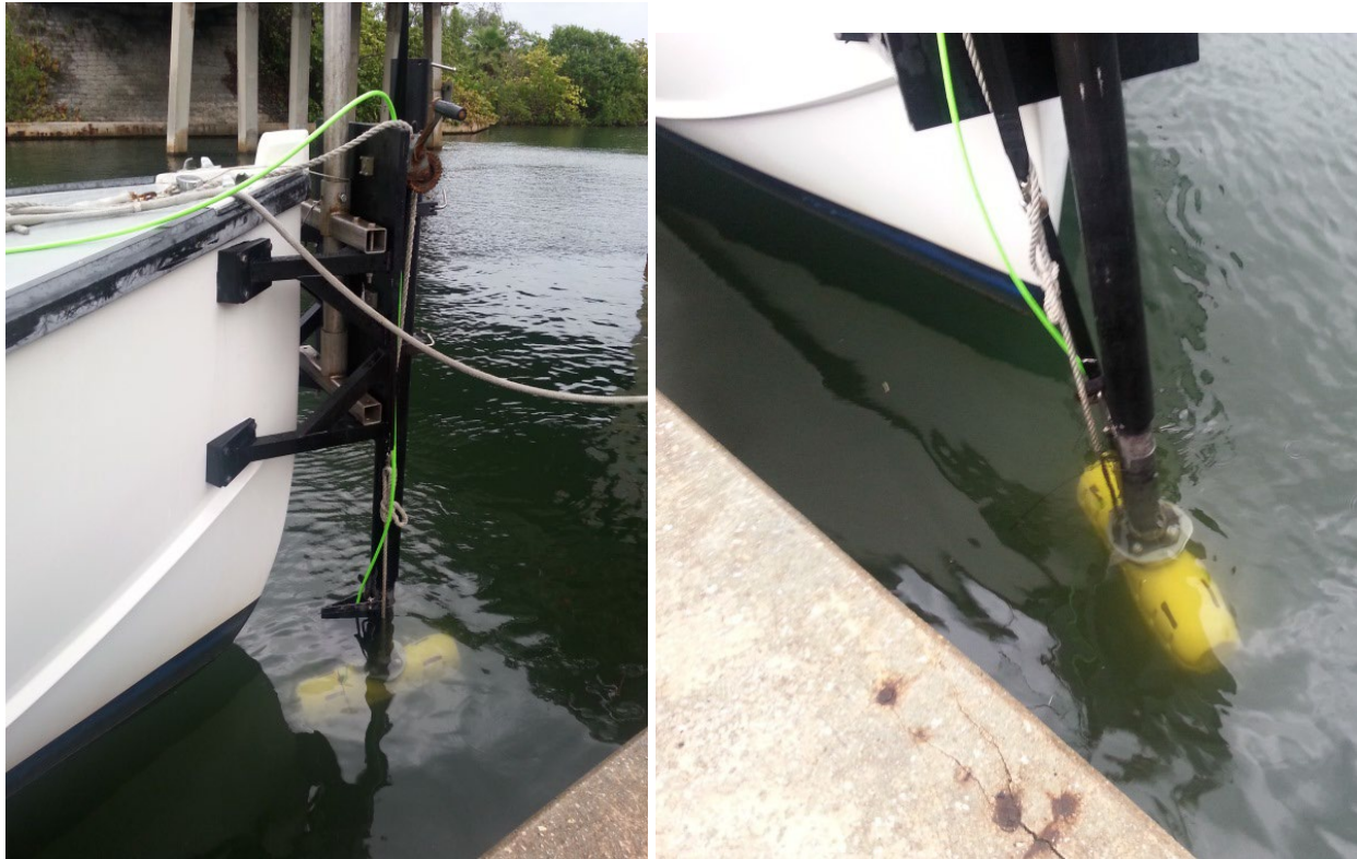
Figure 5-1: 6205s2 Deployment, Option 1 – Over-the-Bow
