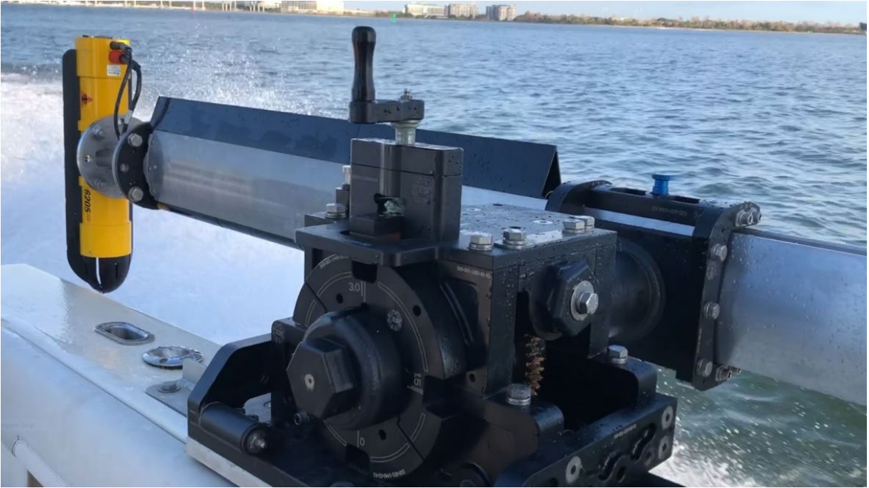
Figure 5-2: 6205s2 Deployment, Option 2 – Over-the-Side
