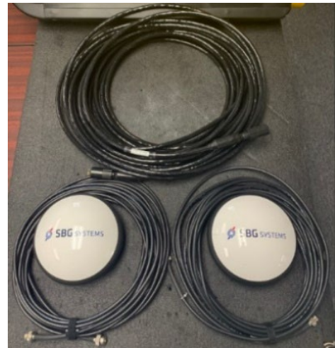
Figure 1-9: GNSS Antenna and Cabling
