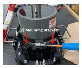
Figure 5-9: 3400 OTS Light and Ultra-Light Transducer Installation - Worm Clamp and Mounting Bracket Locations
