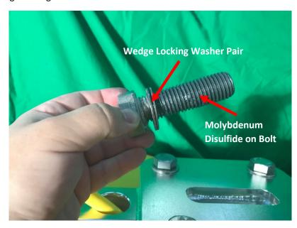
Figure 4-26: Forward Dorsal Bolt Locking Washer and Molybdenum Disulfide Coating
