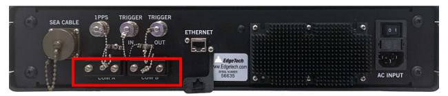
Figure 4-42: 3400 Topside Serial Port Navigation Connection
