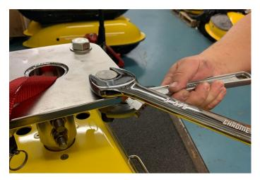
Figure 4-53: 3400 Light and Ultra-Light Adaptor Flange Plate Bolt Assembly - Bolt Tightening
