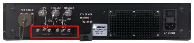
Figure 4-1: 3400 Topside Serial Port Navigation Connection
