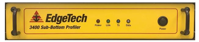
Figure 4-4: 3400 Topside Front Panel-LED Indicator Lights
