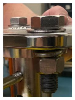
Figure 4-56: 3400 Light and Ultra-Light Adaptor Flange Plate Screw Assembly Locations
