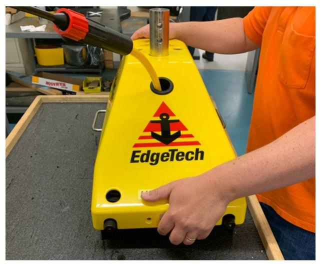
Figure 5-7: 3400 OTS Light and Ultra-Light Shell Removal
