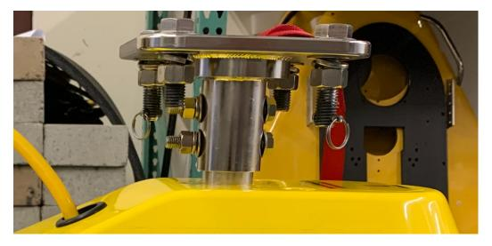
Figure 4-52: 3400 Light and Ultra-Light Adaptor Flange Plate Bolt Assembly Locations
