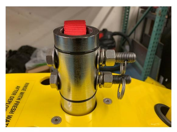
Figure 4-43: 3400 OTS Light and Ultra-Light Pole Mounting with Strap Installed.
