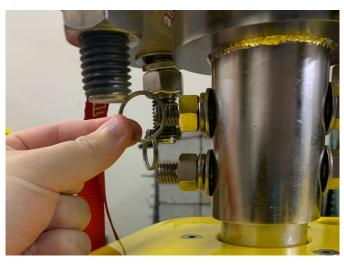
Figure 4-50: 3400 Light and Ultra-Light Adaptor Flange Installation - Split Ring Installation
