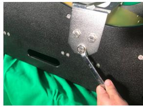
Figure 4-29: Pole Mount Bolt Tightening
