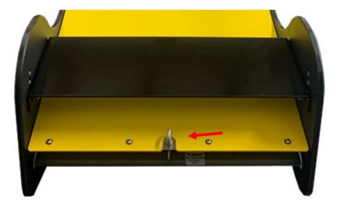
Figure 4-34: Aft Eye Bolt
