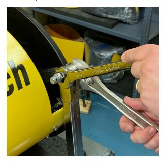
Figure 4-18: Bridle Removal-Elbow Hardware Removal
