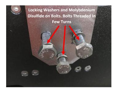
Figure 4-28: Port and Starboard Pole Mount Bolt Positions
