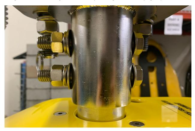
Figure 4-48: 3400 Light and Ultra-Light Adaptor Flange Installation - Bolt Hardware Configuration
