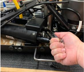
Figure 5-12: 3400 OTS Light and Ultra-Light Electronics Bottle - Mounting Block to Electronics Bottle Mounting Bolt Unthreading
