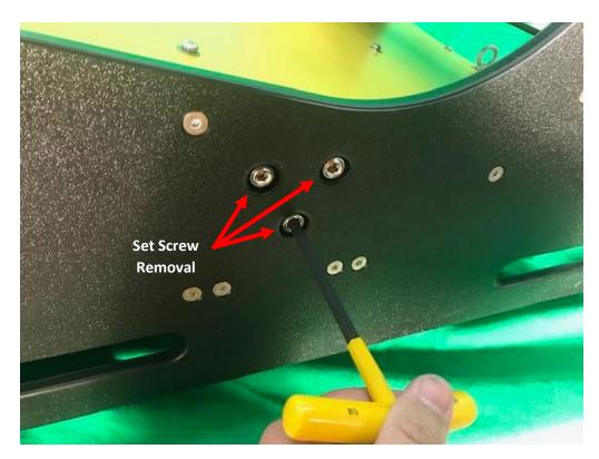
Figure 4-24: Port and Starboard Set Screw Removal
