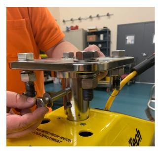
Figure 4-46: 3400 Light and Ultra-Light Adaptor Flange Installation - Threading 1/2" Bolt Assembly
