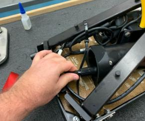
Figure 5-11: 3400 OTS Light and Ultra-Light Electronics Bottle-Cable Disconnection 2
