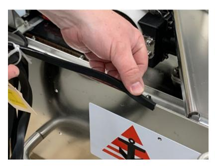
Figure 4-35: 3400 OTS LF Rubber Trim Installation
