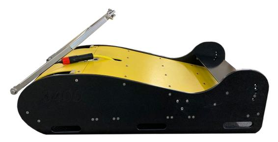
Figure 1-13: 3400 Sub-Bottom Profiler Towfish Port View
