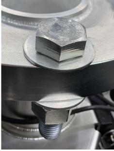
Figure 4-40: OTS LF Mounting Flange with Bolts Installed Figure 4-41: OTS LF Flange Bolt Assembly
