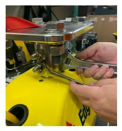
Figure 4-49: 3400 Light and Ultra-Light Adaptor Flange Installation - Tightening Hardware Assembly
