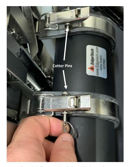
Figure 5-3: Electronics Bottle Cotter Pin Removal
