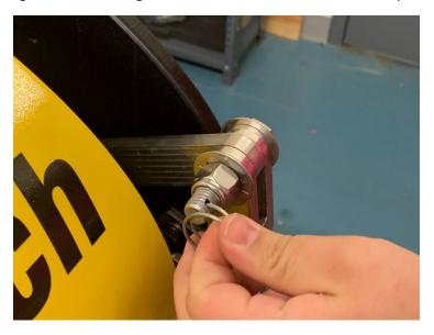
Figure 4-17: Bridle Removal: Split Ring Removal
