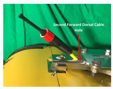
Figure 4-25: Forward Dorsal Pole Mount Cable Hole Position
