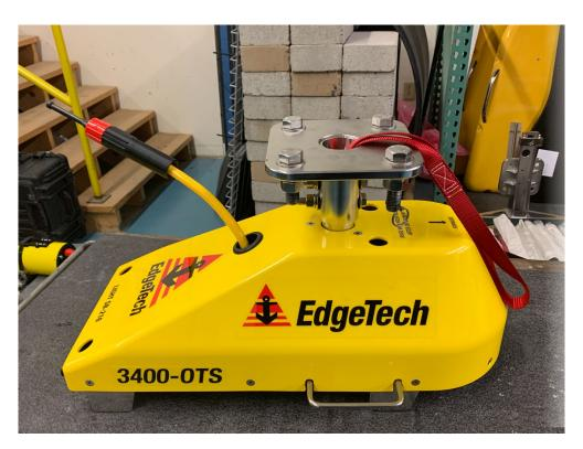
Figure 4-51: 3400 Light and Ultra-Light Adaptor Flange Installation - Pole-Mount Adaptor Flange Mounted
