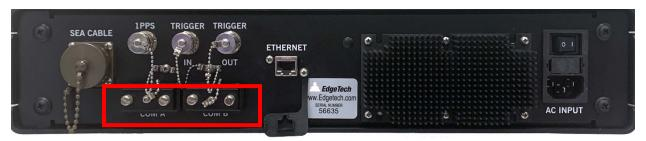
Figure 4-36: 3400 Topside Serial Port Navigation Connection
