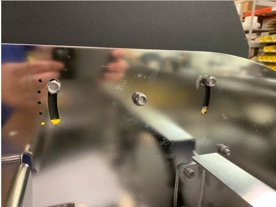
Figure 6-1: View of Inner-Fin Bolt Mounting (Hex Nuts, Washers)
