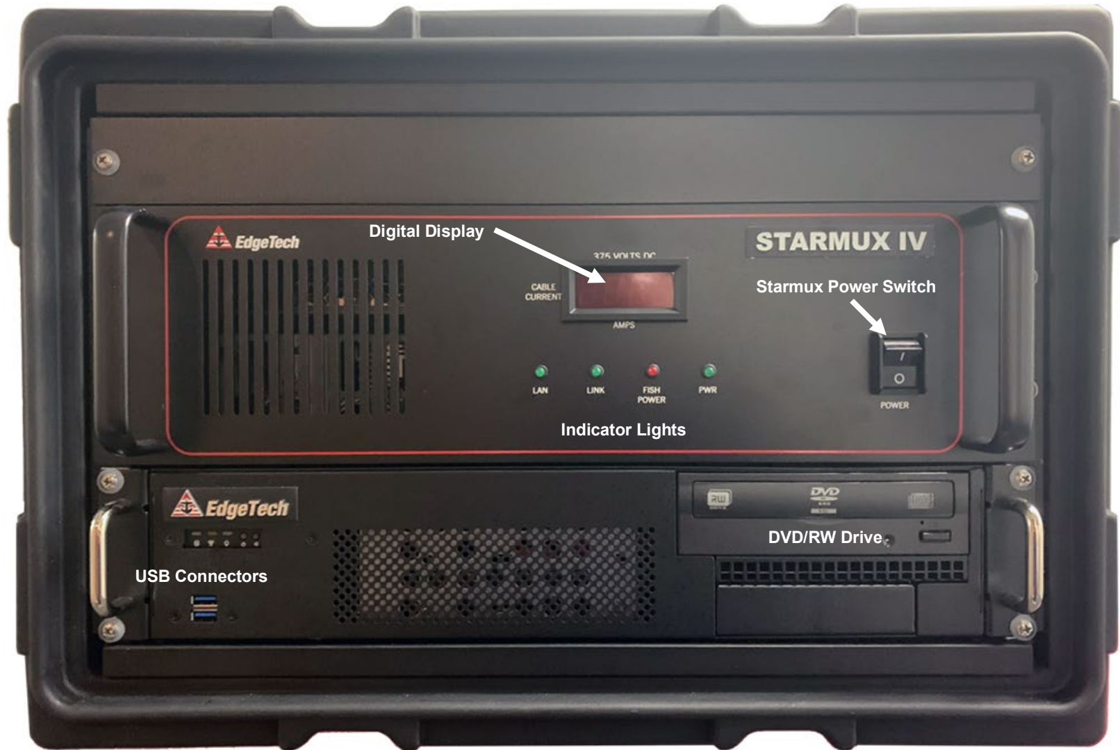
Figure 3-9: Labeled Front Panels of 2300 Rackmount
