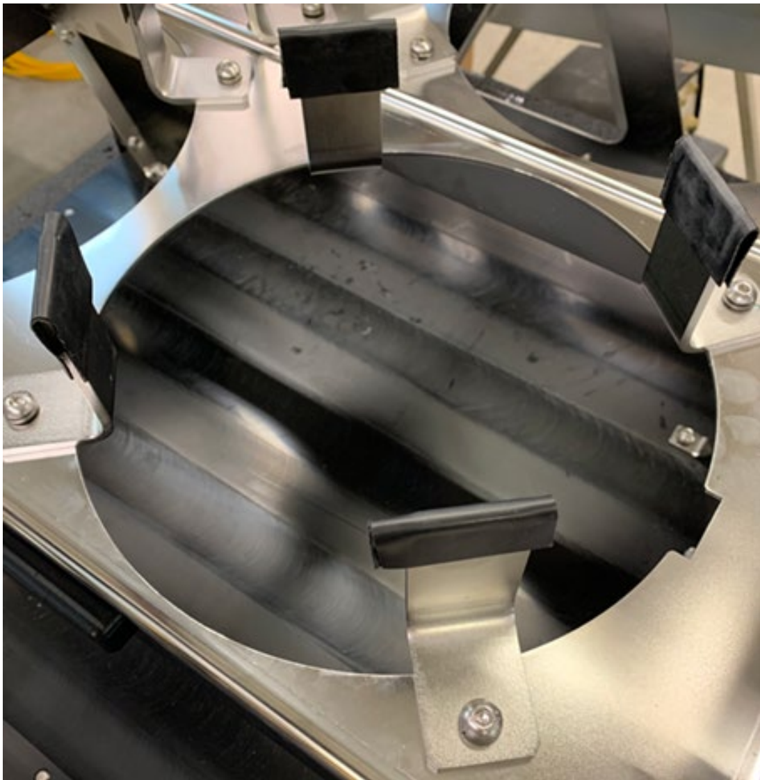
Figure 6-8: Vertical Mounting Brackets Proper Alignment
