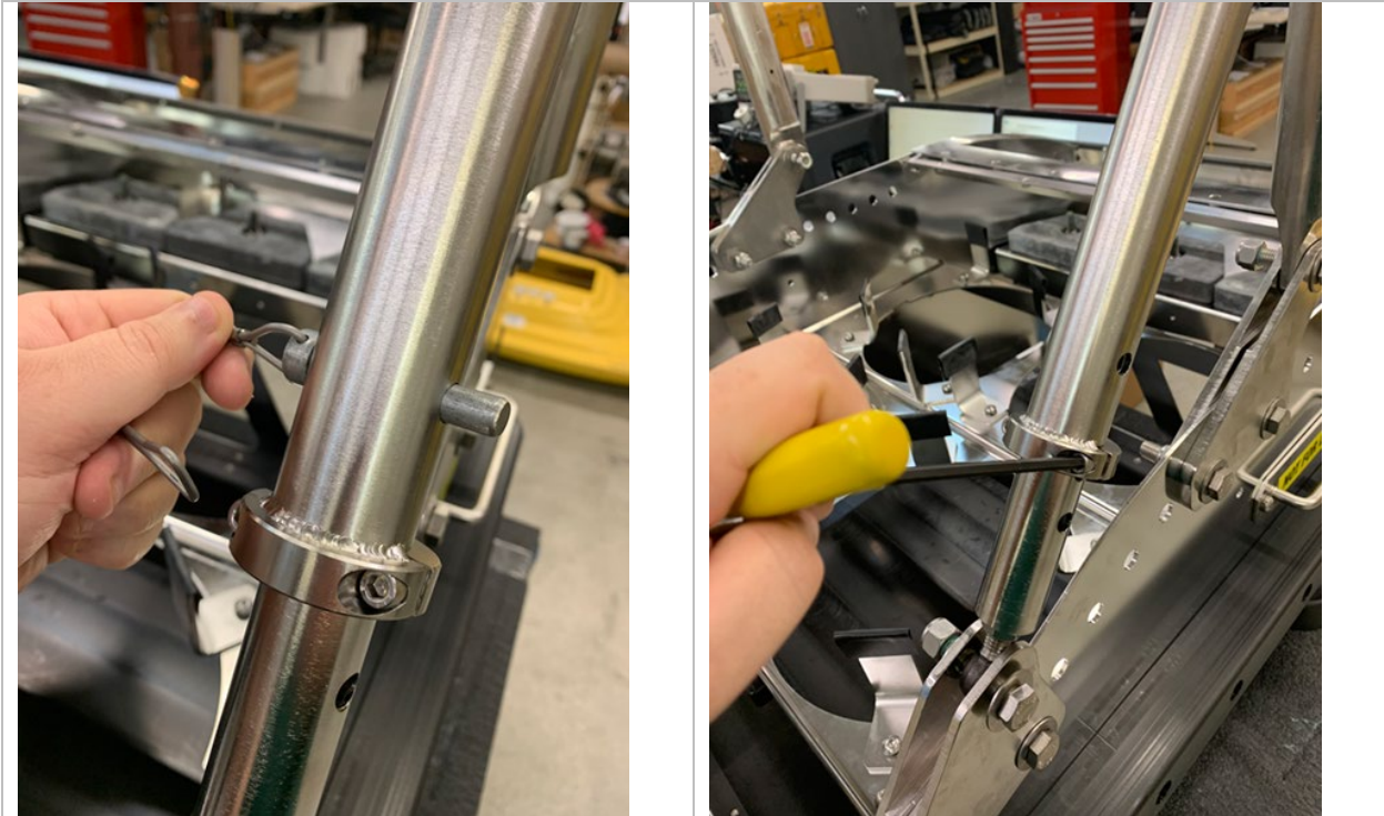
Figure 4-3: Bridle Support Strut Adjustment
