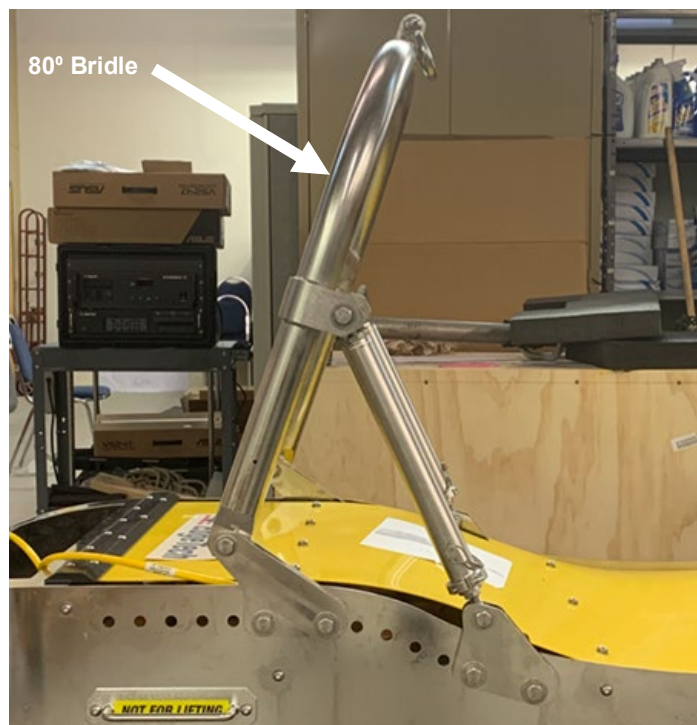
Figure 4-6: Bridle at \sim 80^\circ Position For Crating and Transport
