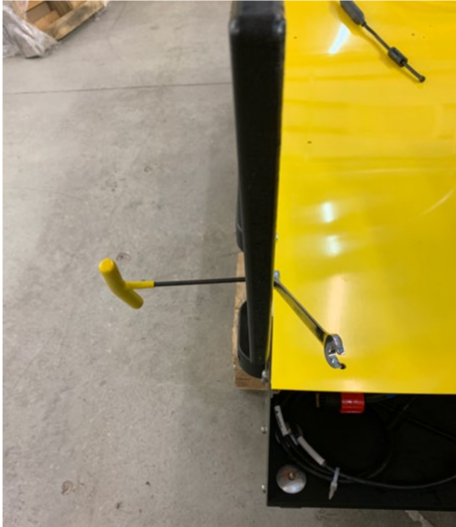
Figure 6-3: Unthreading Tail Wing Assembly with Hex Screwdriver and Wrench.
