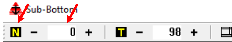
Figure 5-13: Sub-Bottom Shortcut Toolbar- Range Text Field and Normalize Gain Button Called Out
